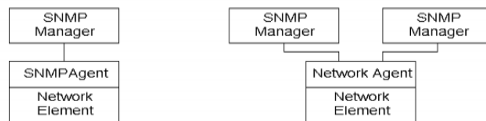
(a) One Manager - One Agent Model (b) Multiple Managers - One Agent Model
