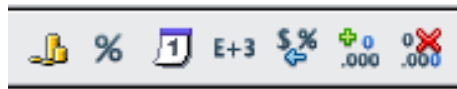
Figure 34: Number format icons. Left to right: currency, percentage, date, exponential, standard, add decimal place, delete decimal place.
