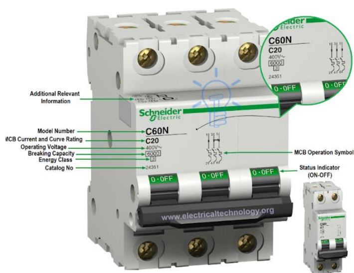
How to Read MCB Nameplate Rating Printed on It
