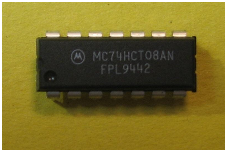
Figure 4-6: 7408 chip, circle indicates top of chip.
