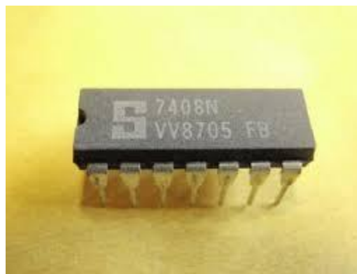
Figure 4-7: 7408 chip, notch indicates top of chip.
